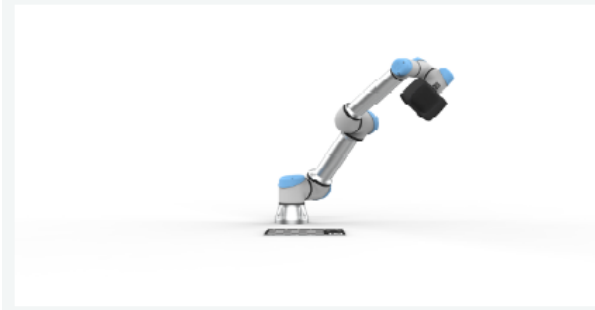
Eye-in-hand robot pose for a close capture of DaoAI calibration board
