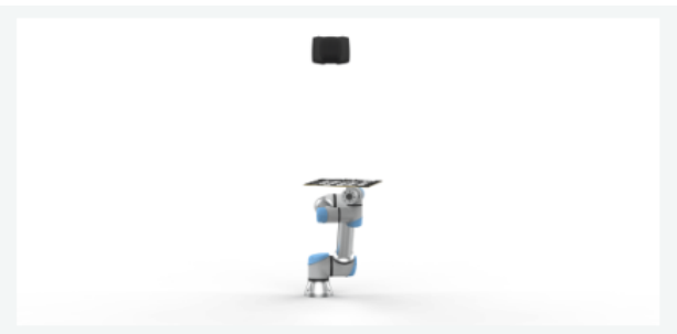
Eye-to-hand robot pose for a close capture of DaoAI calibration board
