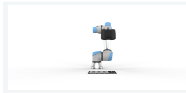
Eye-in-hand robot pose for a close capture of DaoAI calibration board
