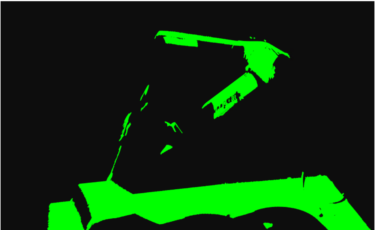
Fig. 15: Point cloud with Remove Small Area
