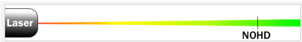
Fig. 1: Color indicates the relative hazard: Red = potential injury, green = unlikely injury. Beyond the Nominal Ocular Hazard Distance, the chance of injury is “vanishingly small” according to safety experts.
